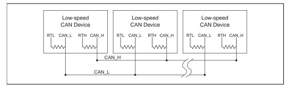
Figure C-4. Termination Resistor Placement for Low-Speed CAN
